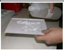
Rinse the moulds with a surfactant mould release and shake dry. An alternative is to use a teaspoonful of dish washing liquid to a litre of water.
