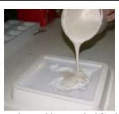
Pour the plaster into the moulds slowly until full. Give the mould several taps to help bring air bubbles to the surface. If overfilled the excess plaster can be removed by wiping over the surface with a flat bladed paint scraper.
