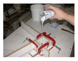
Always ensure before pouring that the mould box is level, using a small spirit level if necessary.
