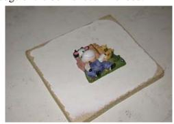
It should be noted that a rolled ribbon of Plastelina pressed around the bottom perimeter of the model works well. The model should be pressed firmly on the base board in all directions. This flattens the clay while at the same time forming a tight seal under the model to prevent rubber from leaking underneath. Remove any Plastelina that is squeezed out past the edge of the model base.
