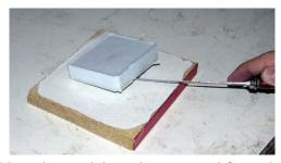
Now the model can be removed from the mould. This is done by gently pushing the silicone away from the model working around the model gradually while getting deeper and deeper until the model is eventually released from the mould.
