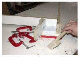
Next break the glue or clay seal between the model and the base board, this is done by inserting a palette knife or flat tool under the silicone, the model and the base. By simply twisting the tool the mould still containing the model is released from the base
