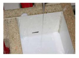
Any air bubbles that rise to the surface can be dissipated by lightly passing an air gun or hair dryer quickly over the surface.
