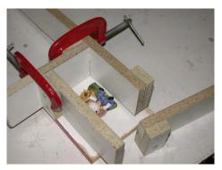
Wood can also be used to make the form when pouring larger moulds. All joints and corners including the area where the walls meet the base must now be sealed with the plastelina non-hardening clay to prevent any possibility of the CraftSil leaking out of the mould box.
