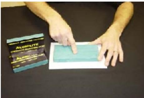
We will start by using a bed of Synthetic Modeling Clay to act as the second half of the mold. Here we have taken a piece of plastic to act as the base of the mold box and are smoothing the bed of clay out to have somewhere to set the original.
