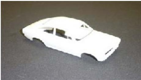
First we will start with an original that requires a two piece mold that will require male and female mold halves. This car works perfectly to demonstrate this because the exterior side will act as our female half of the mold (think of it upside down) and the male (squish) half of the mold will nestle down into the female side to give us the proper part thickness.
