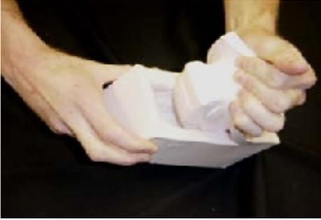
Here you can see the two halves of the mold separating. We wanted to show you this shot, so you can see the advantages of the High Strength 2 flexible silicone rubber with an extremely high tear strength. You will not rip this mold when you demold it. Unfortunately, it is difficult to see the white car body inside the mold. The colors of the rubber and the car are just too close. But the car body remains inside the mold until you flex the bottom half of the mold and remove the original.
