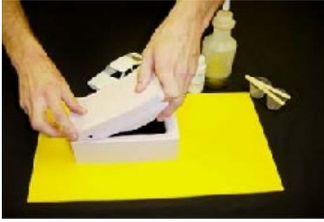
Then starting from the side with the locator, flex the silicone rubber and squish the top half of the mold into the bottom half. Important note: When we use the term squish, we do not mean to apply force. We simply mean to set the male side of the mold into the female cavity to allow the excess resin to be squished out the seam line.
