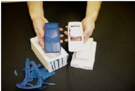
Here is a good picture of the original car along side of our perfectly cast replica. Now all we have to do is to trim out the windows, wheel wells, and bumpers.
