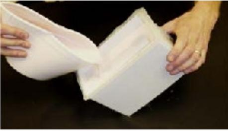
Once you have thoroughly coated the first half of the mold with mold release, you are ready to pour the second half. Mix the High Strength 2 silicone rubber and pour it into the mold box creating the second half of your mold. You can see in this picture we tilted the mold when we began to pour to make sure the silicone got underneath the deep front bumper.
