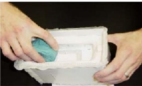
Remove all of the clay from your original. Take the time to remove all of the clay out of the detail of your original ... around the windows, doors, lights, etc. Once you have removed all of the clay you are almost ready to mold release it and pour the second half of the mold.
