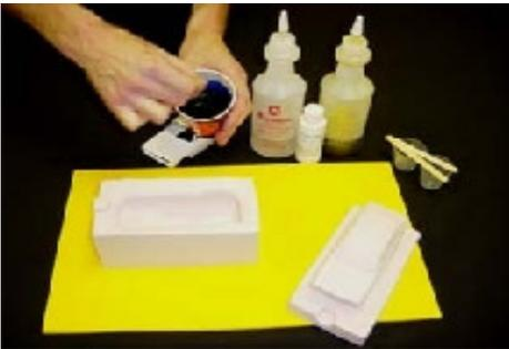
Now we are ready to pour our cast replica. We chose to add some blue dye to the resin to help it show up a little bit better. We simply mix equal amounts of the A side and B side of Alumilite Regular with a few drops of Alumilite's Blue dye. We mixed 2 oz of A and 2 oz of B. Even though the part only requires 2 oz total we use a little more to make sure it squishes properly and pushes all of the air bubbles up and out the seam line.
