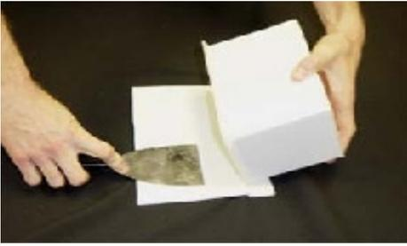
Let the silicone cure overnight. Once cured, using a dull knife or putty knife, remove the mold box from the base.
